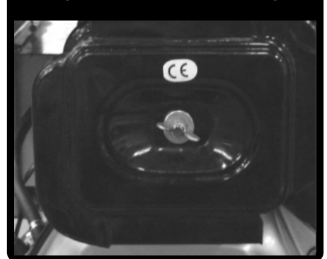
Figure #2 - Air Filter Housing
