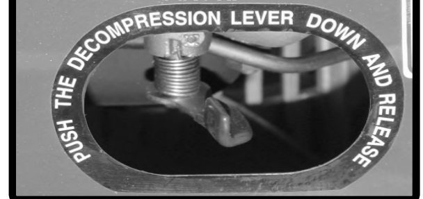
Figure #4 - Compression Release Switch
